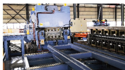
○ 校平机快换辊组 Quick Changing Roll Unit of Leveling Machine
